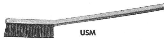
Toothbrush type with straight or offset handles for inking edges, heels and wetting channels. Stiff grey horsehair. Stapled construction.
